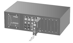
E. Gently push the thumbscrews in and turn clockwise to tighten. *Do not over tighten.*
